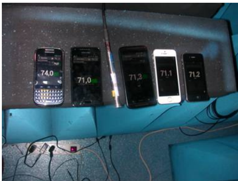
Figure 3. The 5 smartphones and the Class 1 microphone.
