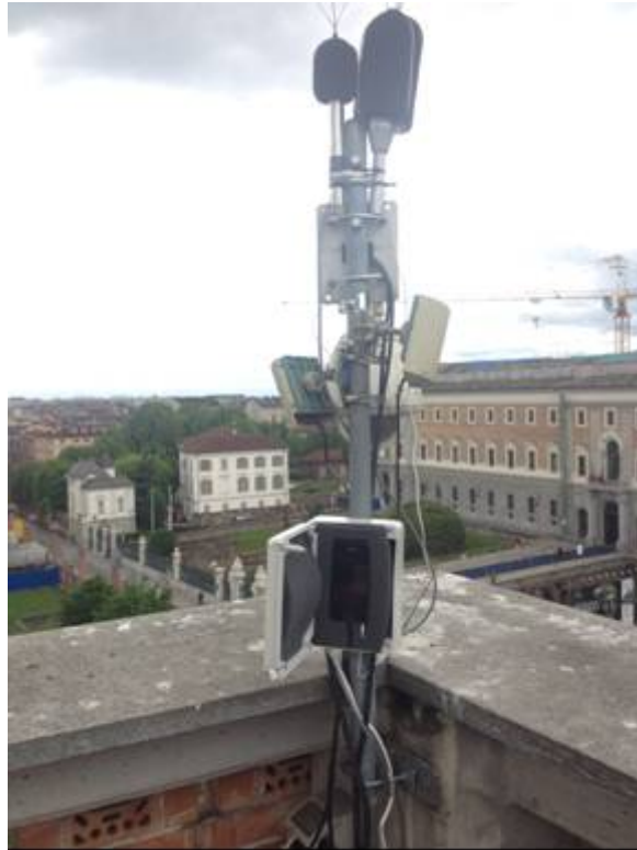
Figure 9. Environmental noise measures on the terrace of a building.
